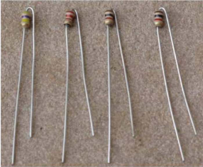
Figure 8. Lead forming for the four resistors. Bend lead tight to the top.
