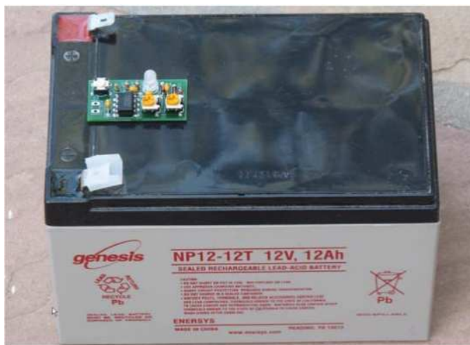
Figure 11. Example of the BSI mounted to the top of a gell cell.
