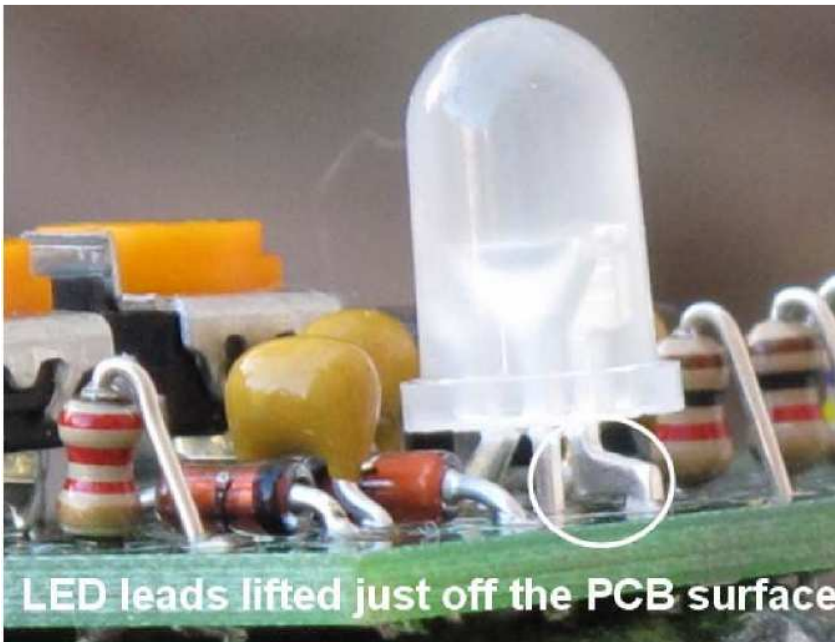
Figure 12. LED leads must be raised just off the surface of the PC board.
