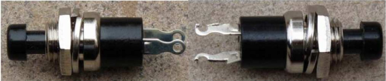
Figure 16. Panel mount push button before and after rework of the switch leads
